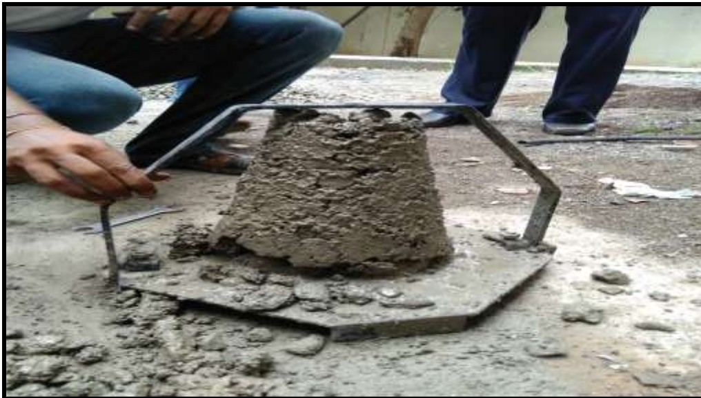
Fig. 2: Slump Cone Testing
